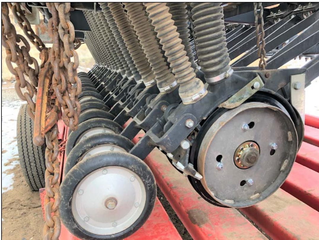
New bearings and disc blades installed on seed drill, January 2020
