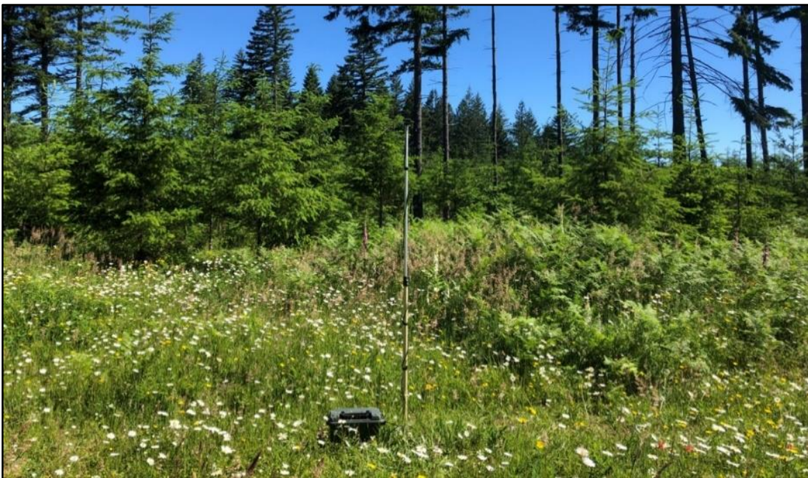
Acoustic bat detector set-up with a microphone on a pole attached to a recording device
