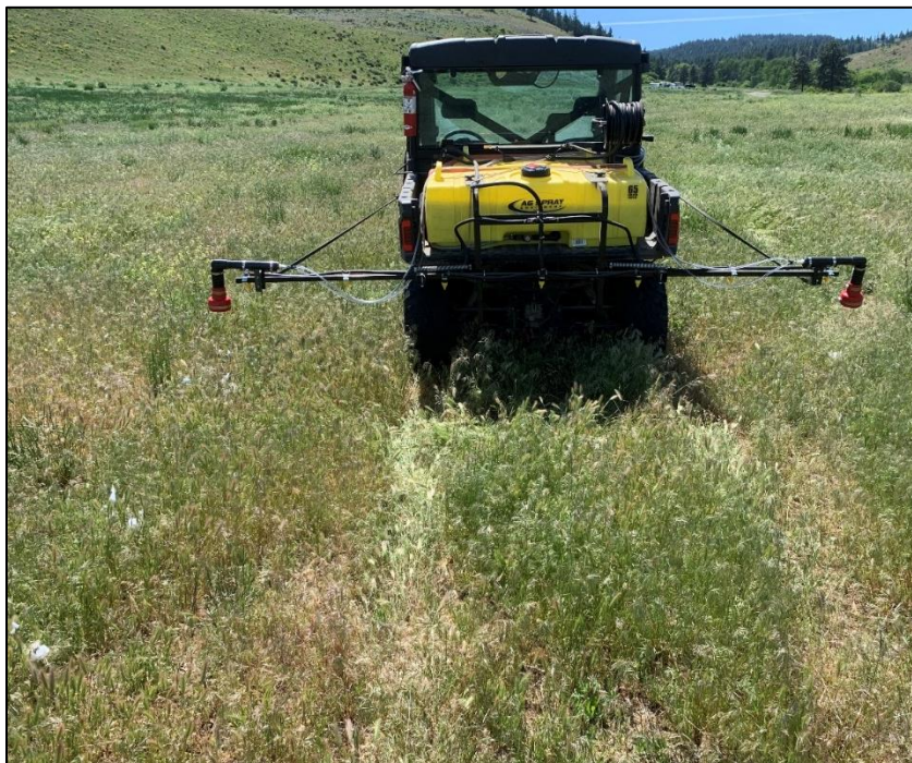
65-gallon spray tank with foam marker at Watt elk feed site
