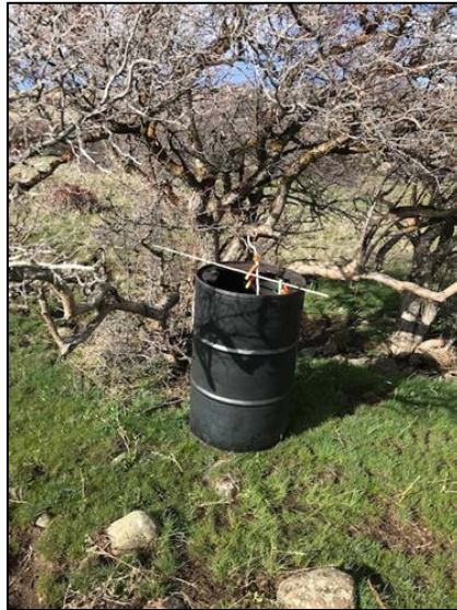
Fused rope in a barrel resonator to deter elk and wolves from irrigated pasture
