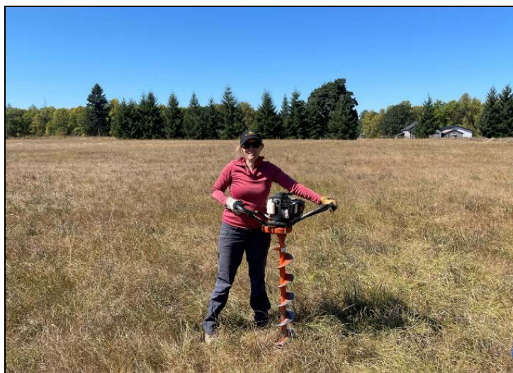
Biologist Butler using a gas-powered auger to take soil samples. Only areas lacking gopher mounds are sampled and samples are taken 6" from surface
