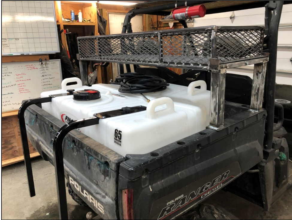
Completed utility box, with newly installed flat bottom sprayer – Photo by Dupont
