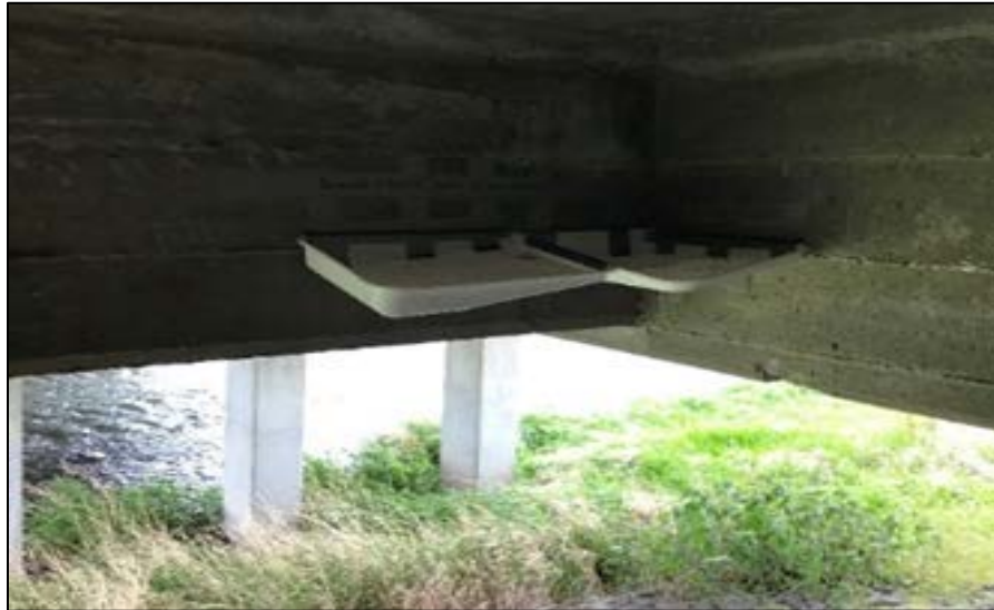
Painter trays mounted to the underside of bridge to collect bat guano for white-nose syndrome surveillance and species identification
