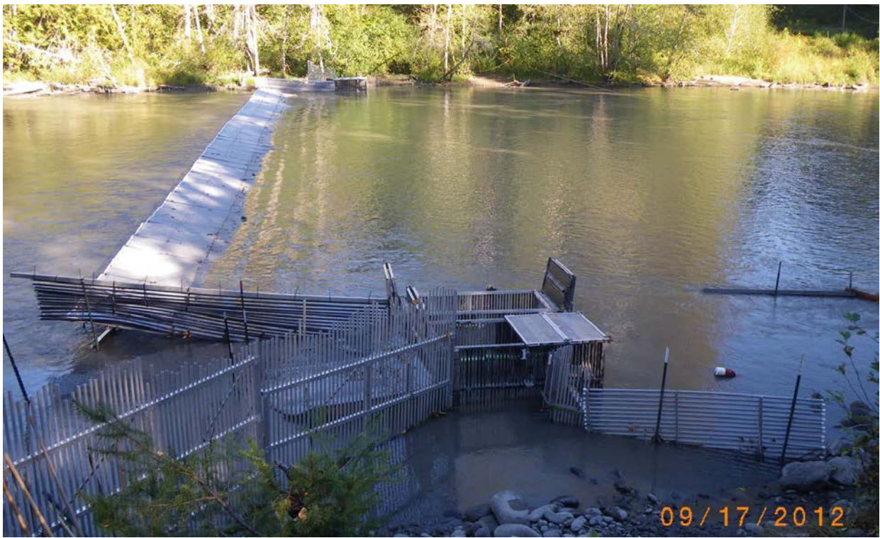
Figure 8. The floating weir in September during the 2012 summer/fall trapping season on the Elwha River. Two upstream traps and two downstream traps were used on river left and river right, respectively.
