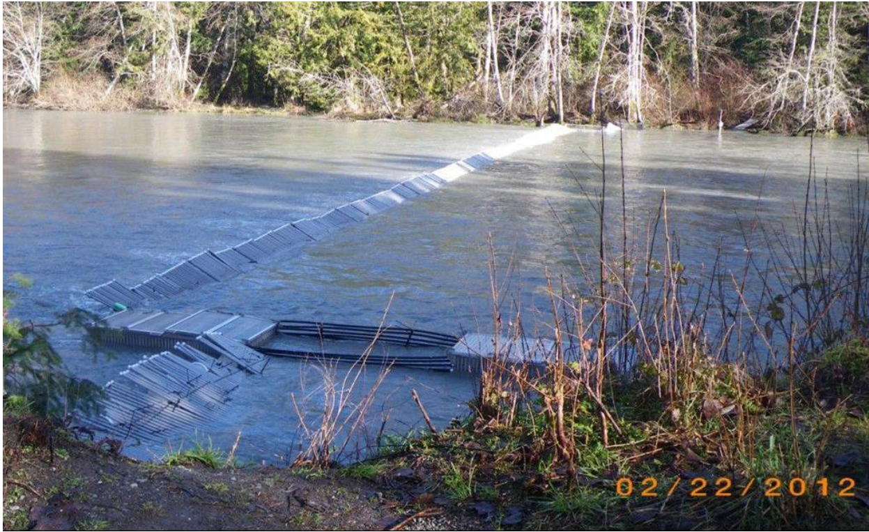
Figure 7. The floating weir fishing at 2,520 cfs during the 2012 winter/spring trapping season on the Elwha River. One upstream trap and one downstream trap on river left (west bank) were used.
